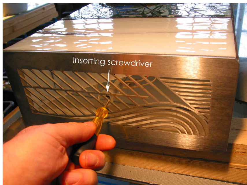
Fig. 7 - Remove the top cover plate (1)
