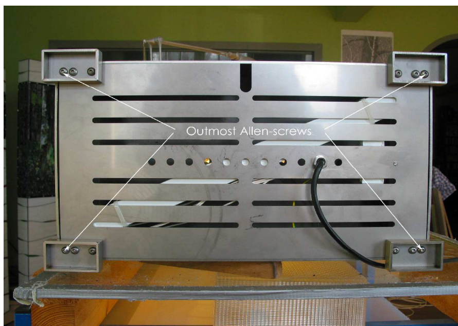
Fig. 14 - Allen-screws to free the pedestal plate
