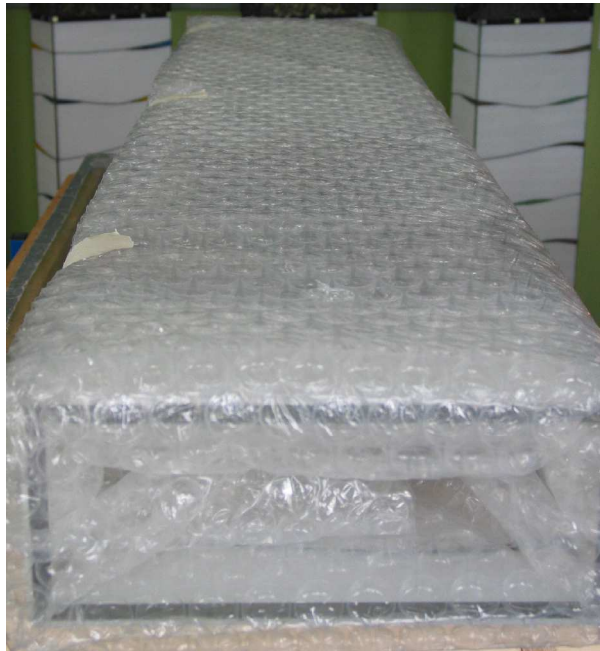
Fig. 16 – Light-column in protective wrap
