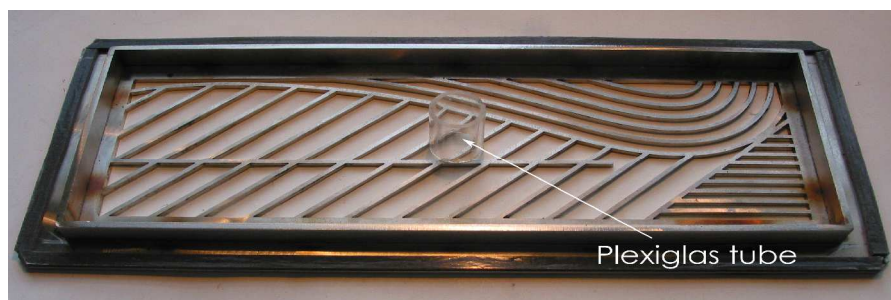
Fig. 12 - Top cover bottom with Plexiglas tube
