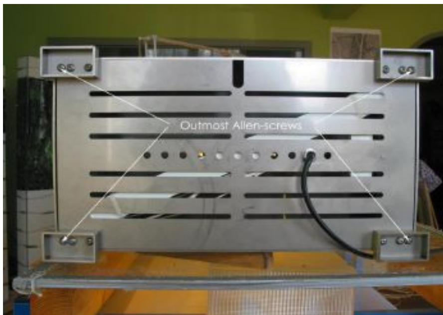
Figure 9 - Allen-screws to free the pedestal plate
