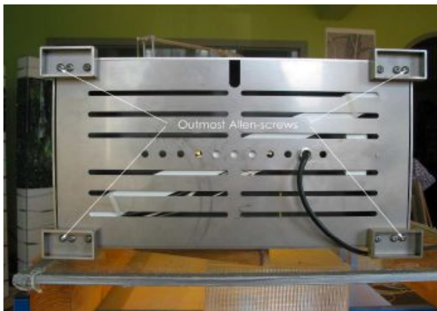
Fig. 14 - Allen-screws to free the pedestal plate
