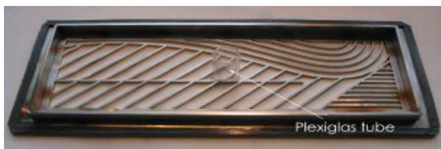
Fig. 12 - Top cover bottom with Plexiglas tube
